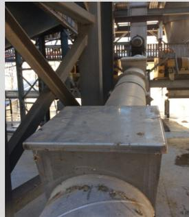
Inspection hatch on a feed mill cross auger. This hatch is not secure and can be lifted off while the auger system is energized.
